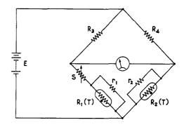
When this bridge is balanced with both thermistors at the same temperature it will remain balanced at any other temperature within the range of linearization provided the temperature of both thermistors remain equal.
