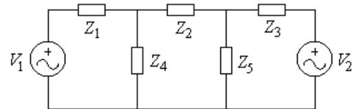
Datos:  $V_1 = 30\text{V}$ ,  $V_2 = 20\text{V}$ ,  $Z_1 = 5\ \Omega$ ,  $Z_2 = 4\ \Omega$ ,  $Z_3 = (2+3j)\ \Omega$ ,  $Z_4 = 5j\ \Omega$ ,  $Z_5 = 6\ \Omega$  y  $f = 50\text{Hz}$ .
