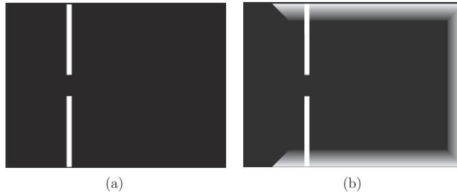
Figure 7. Diffraction by a single slit: (a) density mass and (b) damping maps.
