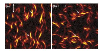
FIG. 1 (color online). Confocal Raman images of SWNT bundles produced by arc discharge on glass acquired by detecting the intensity of the G' band ( $\nu=2615~{\rm cm}^{-1}$ ) while raster scanning the sample (without metal tip, scan area  $15\times15~\mu{\rm m}$ ) for vertical (a) and horizontal polarization (b) of the laser excitation at 633 nm. The arrows indicate tubes which are oriented completely perpendicular to one polarization direction demonstrating the polarization contrast.
