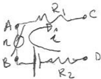
$$V_C - V_D = -R_2 i + V_0 - i n - i R_1 \quad (4)$$
