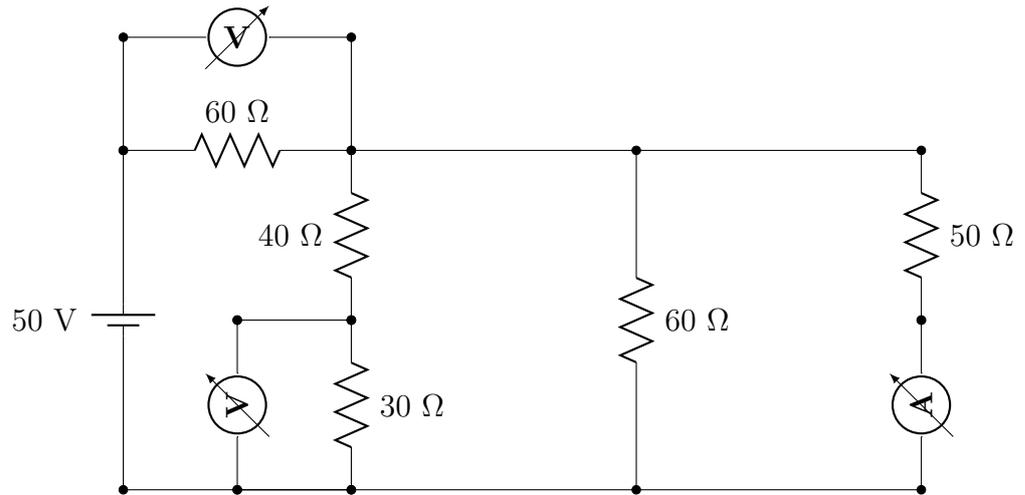
$$R_{70} || R_{60} || R_{50} = \frac{70 \times 60 + 70 \times 60 + 60 \times 50}{70 \times 60 \times 50} = 19.6262 \Omega .$$
