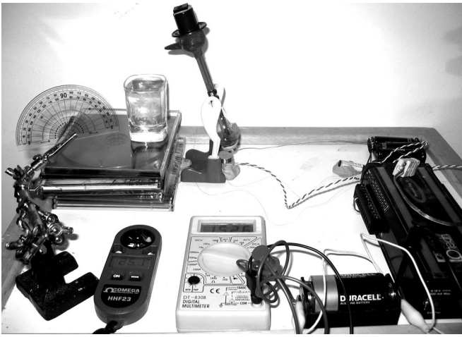
Fig. 1. Experimental setup. A magnet is placed on the base of the bird, just above the coil. Just behind the data logging unit on the right is a small cylindrical magnetometer mounted on putty. The voltmeter in the foreground was used to verify the thermistor excitation voltage. On the lower left is a handheld weather station for recording the temperature and humidity and a protractor mount for calibrating the magnetometer.
