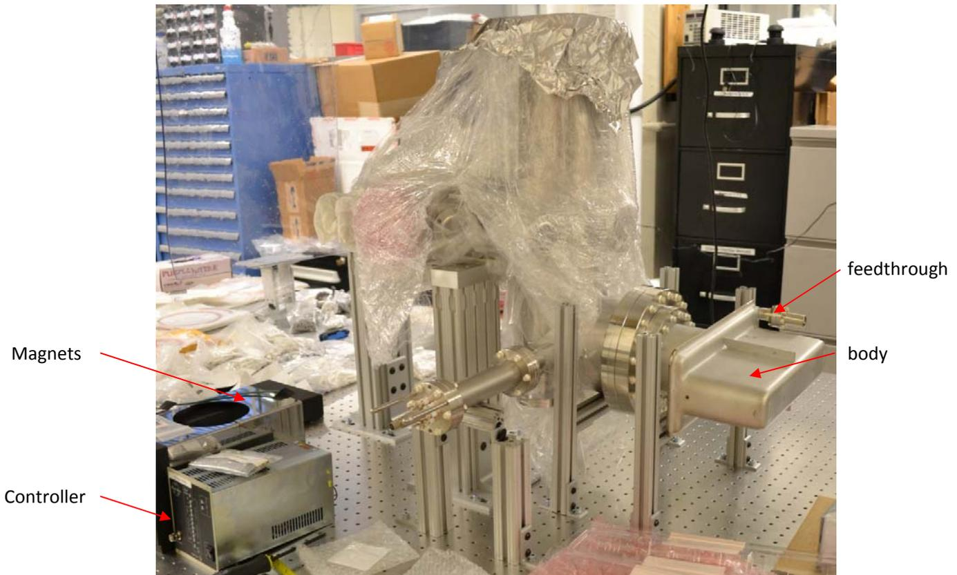
Figure 25. Ion pump mounted.
