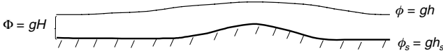
Figure 2.5.1: Schematic of the shallow water model: a hydrostatic, incompressible fluid with a rigid bottom h_s(x, y) , a free surface h(x, y, t) , and horizontal scales L much larger than the mean vertical scale H .
