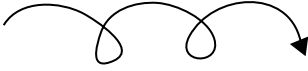
Figure 2.3.1: Schematic of an inertial oscillation in the presence of a basic flow to the right.
