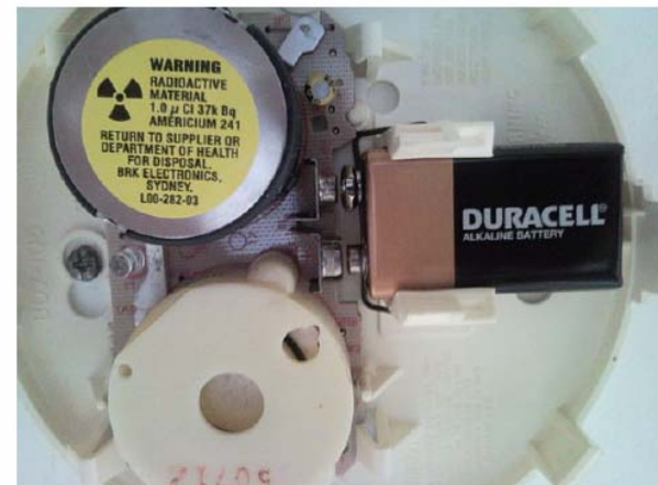
Interior of a smoke detector containing americium-241.
