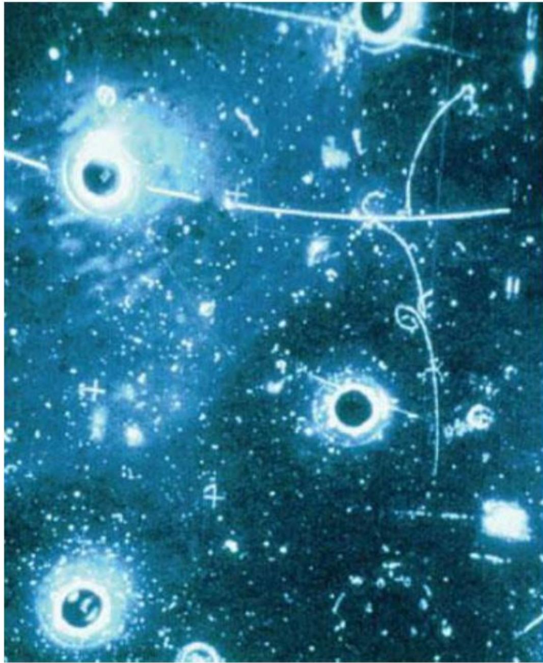
Gargamelle bubble chamber: leptonic neutral current
