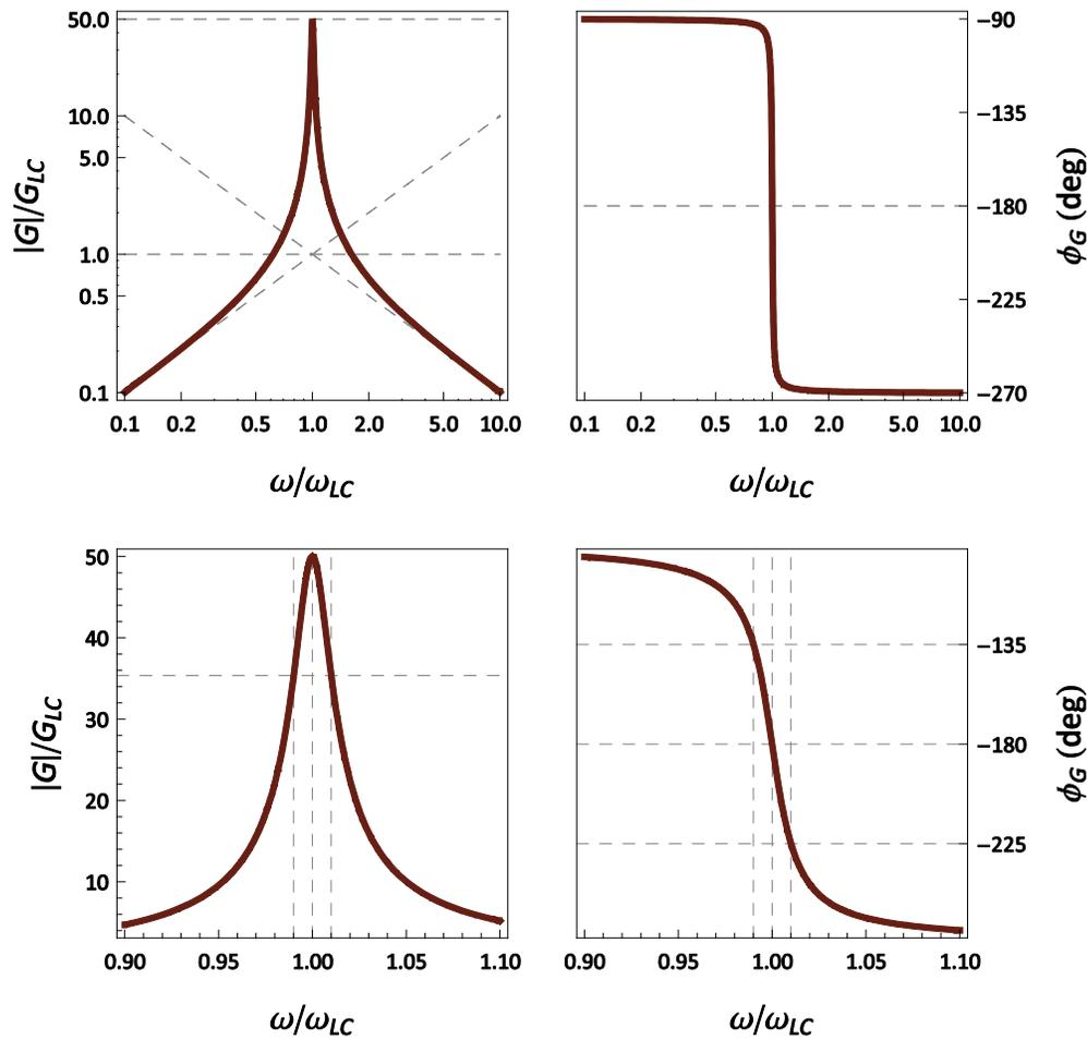
Figure 5-2: Bode plots of the inverting  $LC$  resonant amplifier for  $Q = 50$ . The gain magnitude is normalized to  $G_{LC} = Z_{LC}/R_i$ . Note that the asymptotic gain lines intersect at  $\omega_{LC}$  with  $G = G_{LC}$ , but the actual gain at  $\omega_{LC}$  is  $Q$  times larger. Note that the phase plots have been “unwrapped” so that they remain continuous as the phase passes through  $-180^\circ$  at resonance.
