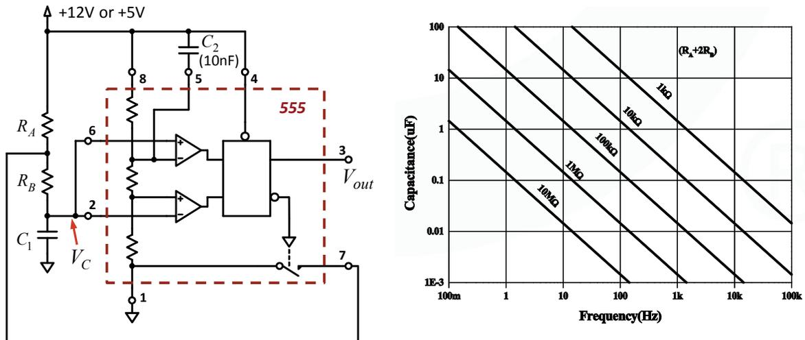
**Figure 4-9: Astable multivibrator using the 555.** The  $V_C$  and  $V_{out}$  waveforms are similar to those for the simple relaxation oscillator in Figure 4-5. Since the capacitor  $C_1$  charges through  $R_A + R_B$ , but discharges through only  $R_B$ , the output waveform is not symmetrical. The graph at right is from the [LM555 datasheet](#); it shows how resistor and capacitor selection affects the output frequency. IC pin numbers are shown next to the 555 terminals in the schematic.
