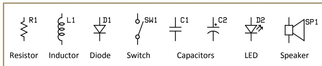
**Figure 1-1: Schematic symbols for a selection of two-terminal, passive circuit elements. Also shown with each symbol is an example of an associated reference designator to uniquely identify that component in a circuit.**
