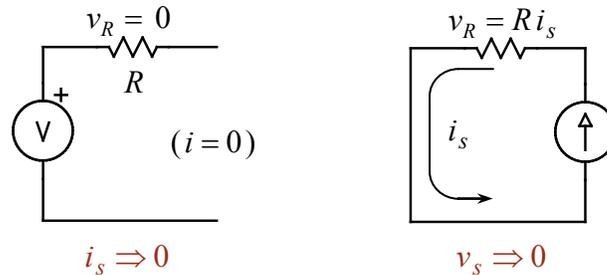
Setting  $i_s$  to 0 (left diagram above) opens the circuit, so no current can flow through  $R$ . Thus  $v_R = Ri = 0$ , and therefore  $(0 = v_R = a v_s) \Rightarrow (a = 0)$ . Setting  $v_s$  to 0 (right diagram) simply connects resistor  $R$  across the current source, so  $v_R = R i_s$ , and  $(R i_s = v_R = b i_s) \Rightarrow (b = R)$ . This gives us the solution for the total voltage across  $R$  due to both sources  $v_s$  and  $i_s$ :
