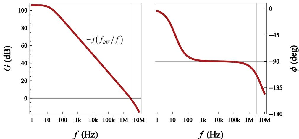
**Figure 2-12: Bode plot of the TL082 op-amp open-loop gain,  $g(\omega)$ . The op-amp’s gain-bandwidth product,  $f_{BW}$ , is 3MHz; the DC open-loop gain is  $2 \times 10^5$ .**
