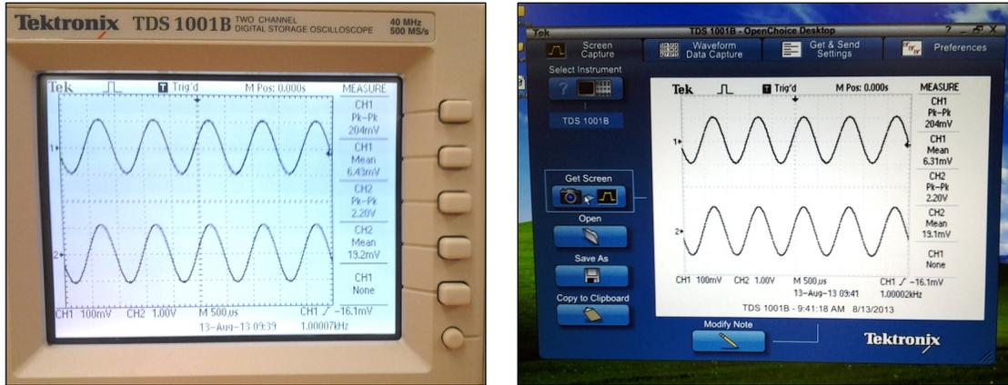
**Figure 1-29: Waveform display using oscilloscope configured to measure input and output signal amplitudes and mean voltages, and a computer screen capture of similar data.**
