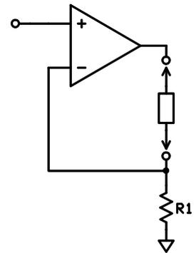
One major drawback of this simple circuit is that the load must be an isolated, 2-terminal device (neither output terminal is a circuit ground, so the load must be able to *float*). We'll investigate transconductance amplifier circuits in a later experiment which relax this requirement.
