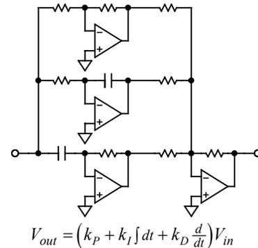
**Figure 7-7: A PID operator circuit commonly used to process an error signal. The weights of the individual terms may be adjusted by selecting appropriate values for the input resistors in the final summing amplifier.**
