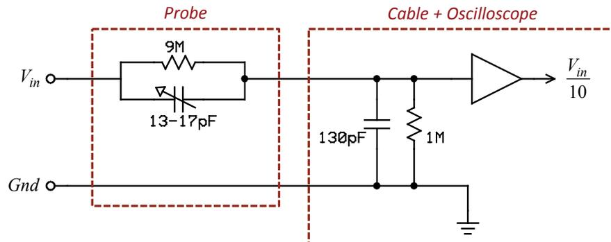
**Figure 2-22:** Schematic of a 10x oscilloscope probe connected to an oscilloscope input channel. The adjustable probe compensation capacitor keeps the voltage divider ratio at 10:1 at all frequencies, even in the presence of the large input + coaxial cable capacitance ( $130\text{pF}$ ). The equivalent input impedance at the probe tip is  $10\text{M}\Omega$  in parallel with about  $13\text{pF}$ .
