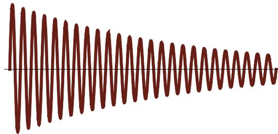
Figure 5-3: First 25 cycles of the output ringing of the circuit in Figure 5-1 for  $Q = 50$ . A negative step in the input would excite this response; the ringing initial amplitude would be approximately  $Z_{LC}/R_i$  times the input step amplitude.
