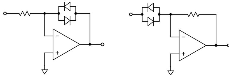
**Figure 3-7: Inverting log (left) and exponential (right) circuits using diodes. These simple circuits are not very accurate and are very temperature-sensitive, but will work for noncritical applications. The paralleled back-to-back diodes will treat positive and negative input voltages the same, using whichever diode is forward-biased to dominate the circuit transfer function.**
