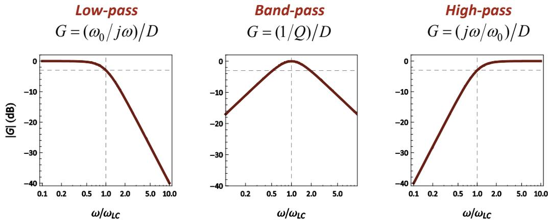
Figure 5-11: Transfer functions and Bode gain plots for the second-order filters of Figure 5-10 for  $Q^2 = 1/2$ . The  $-3\text{dB}$  gain points for the band-pass filter are at  $0.52\omega_0$  and  $1.93\omega_0$ ; for the others it is at  $\omega_0$ . The out-of-band filter slopes are  $\omega^{-2}$ ,  $\omega^{+1}$ , and  $\omega^{+2}$ . The denominator  $D$  in the gain formulas is defined in equation 5.7.
