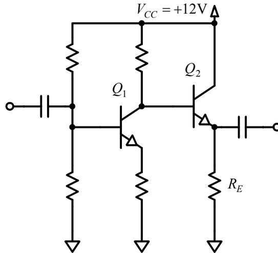
**Figure 6-11: Adding an emitter follower output stage to the common emitter transistor amplifier circuit. The added components are transistor  $Q_2$  and its emitter resistor  $R_E$ . The output coupling capacitor is moved from the collector of  $Q_1$  to  $Q_2$ 's emitter.**
