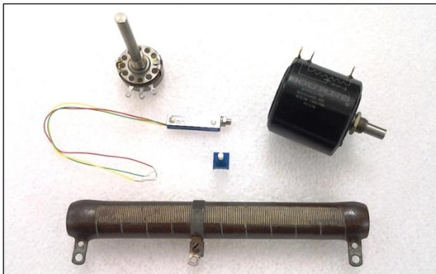
Figure 1-8 (left): A selection of potentiometers. All except the one at the bottom of the photo are adjusted by turning a shaft. The bottom device clearly shows how a potentiometer is constructed, in this case from a long coil of high-resistivity wire, such as nichrome. The two ends of the resistive element are attached to terminals on the device; the adjustable wiper contact is attached to the remaining terminal.
