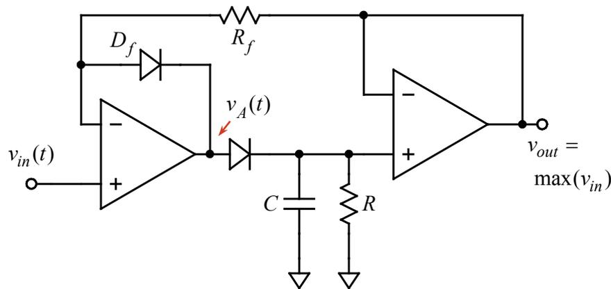
**Figure 3-16: A modified peak detector with improved frequency response. The feedback loop now comes from the voltage follower output; the addition of  $R_f$  and  $D_f$  ensures that the loop stays closed when  $v_{in}$  drops below  $v_{out}$ . Now the first op-amp output ( $v_A$ ) never gets further than a diode drop away from  $v_{in}$  while it is below  $v_{out}$ , rather than saturating at its negative limit as is the case in the Figure 3-15 design.**
