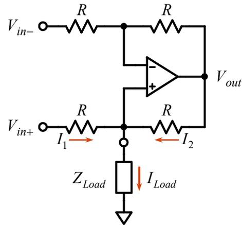
inverting amplifier with  $V_{out} = -V_{in-}$ . Now the voltages  $V_{in+}$  and  $V_{out}$  appear across the resistances  $R$ , determining currents  $I_1$  and  $I_2$ . Thus the load current is given by:
