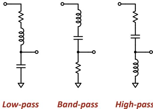
**Figure 5-10:** Series  $LCR$  circuits configured as simple filters. By forming a voltage divider and taking the output from the voltage across each of the various elements, various filter responses may be achieved. In each case the resonant frequency is, of course,  $\omega_0 = 1/LC$ ; the quality factor  $Q = Z_{LC}/R$ .
