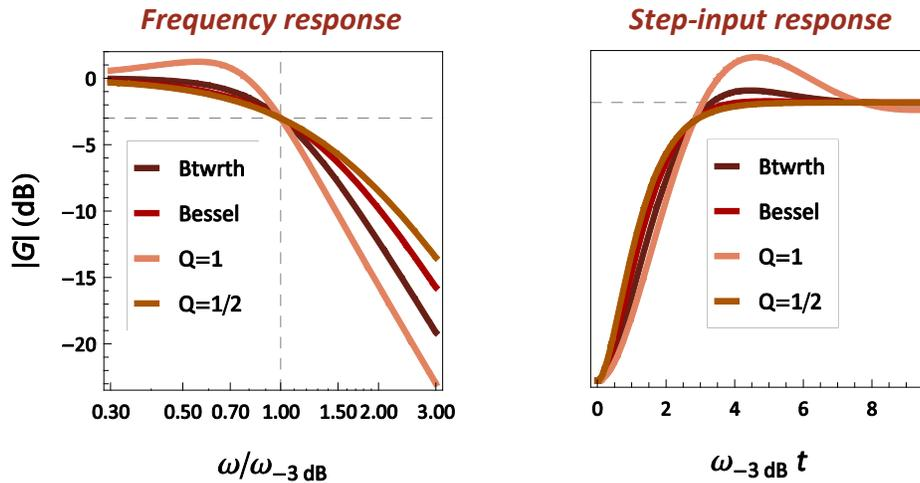
**Figure 5-12: Frequency and transient responses of various 2<sup>nd</sup> order low-pass filters. All filters have the same  $-3\text{dB}$  frequency, but have different  $Q$ 's (the Butterworth filter has legend "Btwrth"). The critically damped filter has  $Q = 1/2$ . The  $Q = 1$  filter has mild gain peaking ( $+1.25\text{ dB}$ ), but significant step response overshoot; its resonant frequency is  $0.79$  of its  $-3\text{dB}$  corner frequency.**
