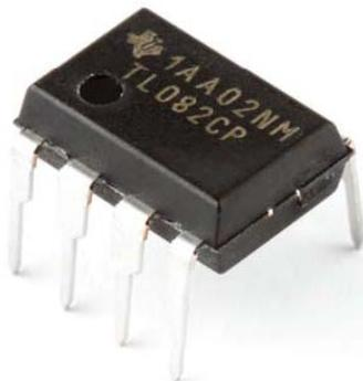
**Figure 1-13:** A photo of an IC operational amplifier, the Texas Instruments Inc.'s TL082 device. This integrated circuit is the type you'll use for your circuits in this experiment; it actually contains two independent op-amps in the package shown (called an 8-pin *DIP*, for "dual-inline package"). The spacing of the connector pins in one row is 0.10inch (2.54mm); the two rows are 0.30inch apart. (Photo courtesy Texas Instruments Inc., ©2012)
