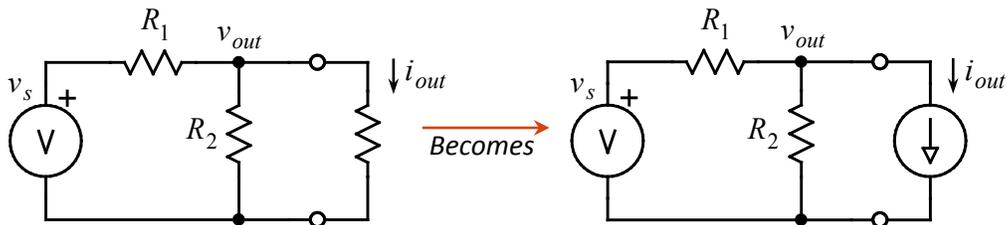
Figure 1-35: Determining the output resistance of a voltage divider driven by an ideal voltage source. Think of the load as a *current sink* (right schematic) and then set the source to 0; this puts the two resistors in parallel, and that parallel combination gives the output resistance,  $r_{out}$ .
