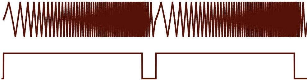
**Figure 7-1: Sample output of the *swept-frequency function generator*. Top trace: generator output sweeping up through a 10-fold frequency range and then rapidly resetting to its original frequency and repeating (triangle output shown, but a sweeping square output should be available as well). Bottom trace: the accompanying “sync” signal which could be used to synchronize an oscilloscope to the output sweep.**
