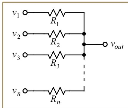
**Figure 1-22: A generalization of the voltage divider circuit. Several voltage sources are connected to a single node via resistors, and we want to know the resulting voltage at that node ( $v_{out}$ ).**
