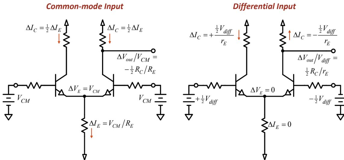
**Figure 6-15: Responses of the differential amplifier stage to common-mode (left) and differential (right) inputs. The currents and voltages shown are the changes to the quiescent operating state values shown in Figure 6-14.**
