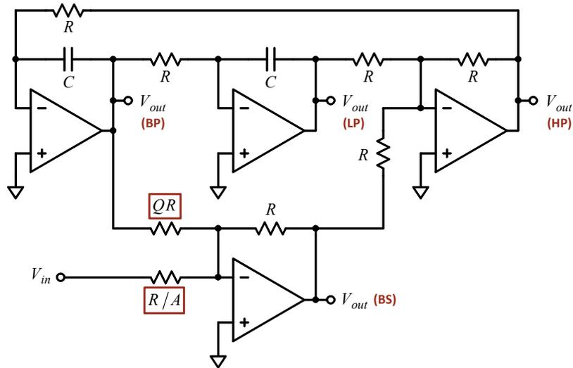
Figure 5-16: A *Universal Active Filter (UAF)*, a form of second-order, state-variable active filter. This design is from the [Texas Instruments ASLK Pro Manual](#), ©Texas Instruments, 2012. It simultaneously provides high-pass (HP), low-pass (LP), band-pass (BP), and band-stop (BS) outputs. The pass-band filter gain is  $A$ ; its resonant frequency is  $\omega_0 = 1/RC$ .
