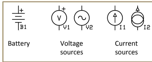
**Figure 1-2: Schematic symbols for common voltage and current sources; each is a two-terminal, active element. Polarity or current flow has the direction indicated when the source output is positive. The battery symbol will often be used to represent any constant-voltage (DC) source such as a power supply. The other sources may be constant or time-varying (an “AC source” usually means that its output varies sinusoidally –  $\sqrt{2}$  in the figure represents an AC voltage source).**
