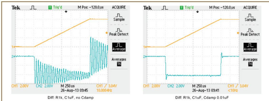
Figure 2-18: Undamped (left) and damped (right) differentiator responses to a sudden change in input slope. The input slope transitions between 0 and 4V/ms; the output should change between 0 and -4V ( $RC = 1\text{ms}$ ). In the damped case  $C/C_{damp} = 100$ , resulting in a not quite critically damped response, with about a 10% overshoot and about 1 resonant cycle required to reach steady state.
