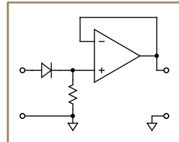
Again using a silicon diode, replace the simple half-wave rectifier circuit with a precision version (Figure 3-4). Examine the output and note that the 0.6V diode drop is no longer evident. Compare your results to Figure 3-6.
