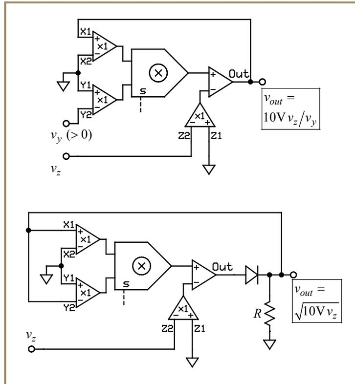
You must always provide negative feedback for the output op-amp of the MPY634. Any unused differential input terminals must be connected to ground.
