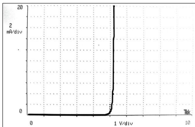
**Figure 3-17: Measured Zener diode I-V curve. The reverse diode current is plotted as a function of the applied reverse-bias voltage. As the applied voltage exceeds 5V, the diode current dramatically increases as the diode suffers reverse breakdown. As can be seen from the plot, diode reverse currents above about 15 mA correspond to a reverse-bias voltage of 5.3V. A lab instrument called a *curve tracer* was used to perform this measurement (Tektronix 571).**
