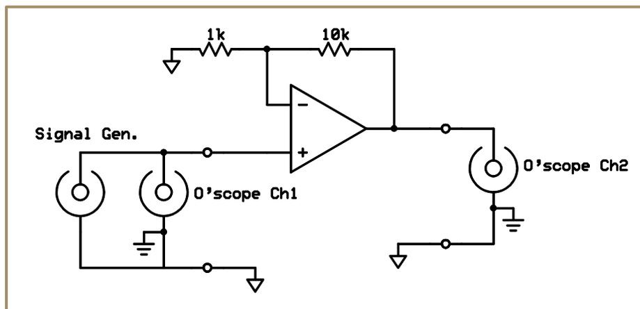
**Figure 1-28:** The first circuit you should build, which is shown in Figure 1-26 as well. Note that the oscilloscope's internal connections of its BNC shells to *Earth Ground* are also shown.
