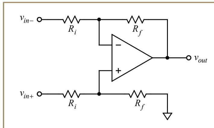
**Figure 1-20: The Differential Amplifier.** The added voltage divider on the  $v_{in+}$  input will divide it by just the right amount so that the output is proportional only to the *difference* between the two input signals, equation 1.8.
