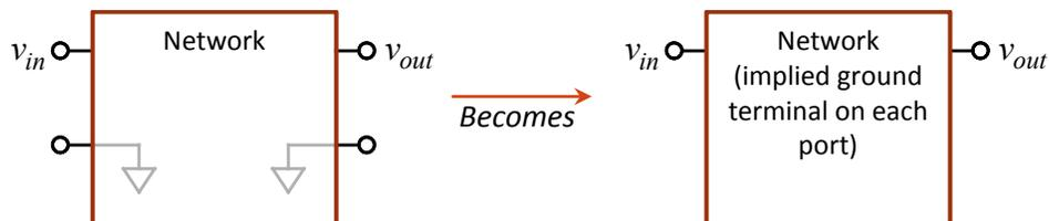
**Figure 1-12: A network whose ports each use *ground* as one terminal. In this case the ground terminal is often not shown explicitly, so only a single terminal is shown for such a port. Since ground is our circuit’s 0-Volt reference, the voltage of the single terminal is sufficient to determine the voltage of the port.**
