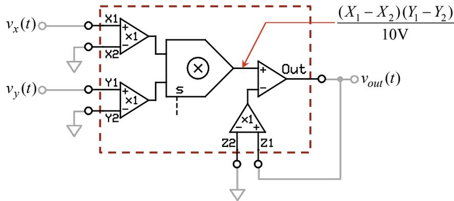
**Figure 3-11: Functional block diagram of the Texas Instruments MPY634 analog multiplier. Besides the basic multiplier, the IC includes a general-purpose op-amp on the multiplier's output and has differential inputs for all parameters, including the Z inputs to the op-amp's feedback (-Input) terminal. Shown in light gray are the connections needed to emulate the basic generic multiplier discussed in the previous section.**
