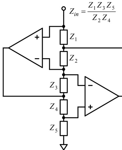
Figure 5-7: A practical gyrator circuit. The op-amps will maintain their inputs at the same potential, so the voltage across  $Z_5$  and the voltage at the junction of  $Z_2$  and  $Z_3$  must both equal the input voltage. With this condition it is straightforward to derive the input impedance formula shown.
