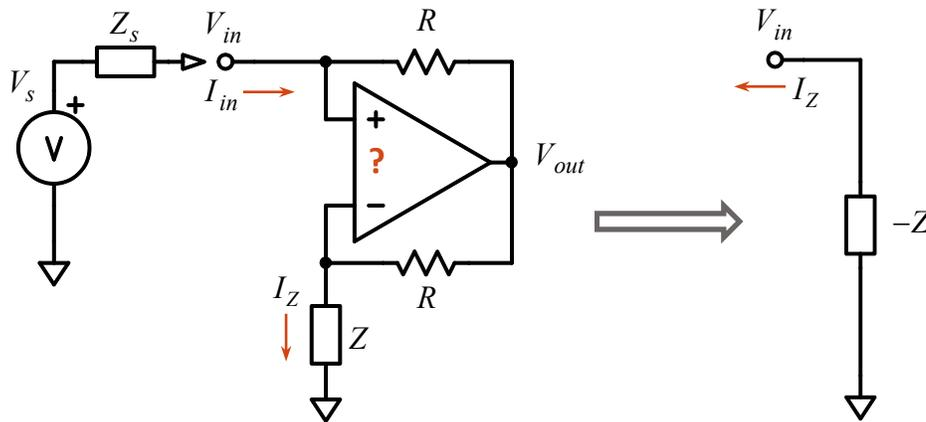
**Figure 5-5: A negative impedance circuit.** As explained in the text, the input impedance of the op-amp circuit,  $V_{in}/I_{in}$ , is  $-Z$ , the *negative* of the impedance of the element  $Z$  in the circuit. The “?” on the op-amp symbol implies that we must carefully consider how the op-amp's inputs should be connected — with *-Input* at top as shown, or should the op-amp's inputs be flipped? This issue is discussed in the text.
