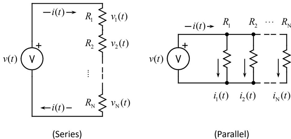
**Figure 1-6: Series and parallel resistor combinations.** For the series case, the same current flows through all resistors, and the total voltage is the sum of the individual resistor voltages. For the parallel case, the voltage is the same across all resistors, whereas the total current from the source is the sum of the individual resistor currents. The results are that series resistances add; parallel conductances ( $1/\text{resistance}$ ) add.
