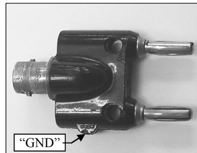
Figure 1-27: BNC adapter showing the tab identifying the connection to the BNC shell.
