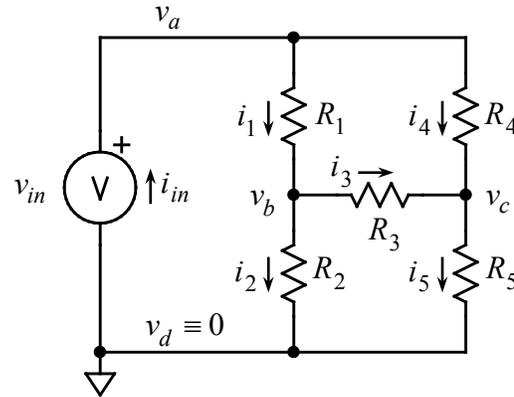
**Figure 1-34:** A nontrivial example to exercise the circuit voltage and current rules: a resistor “bridge” with voltages and currents identified and labeled for analysis. The bottom node is defined to be ground, so the voltage there is 0 by definition. The source is assumed to supply voltage  $v_{in}$ , and the circuit draws current  $i_{in}$  from it.
