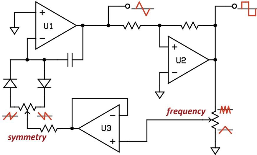
**Figure 4-7: A function generator circuit with variable frequency and waveform symmetry. The voltage follower using op-amp U3 isolates the Schmitt trigger output and the frequency adjust potentiometer from the current load demands of the integrator, especially important when the symmetry potentiometer is set near one of its limits.**
