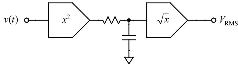
The scale factors of the multipliers used for the square and square root circuits don't matter as long as they are the same; Figure 3-12 shows a square root circuit using the MPY634.
