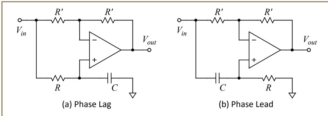
**Figure 2-23: Unity-gain phase shifters (all-pass filters).** Although  $|V_{out}/V_{in}| = 1$  at all frequencies, the phase of the output decreases through  $180^\circ$  as frequency goes from low to high. In the circuit (a) the phase at low frequency is  $0^\circ$ , but lags through  $-90^\circ$  at  $f = 1/(2\pi RC)$  toward  $-180^\circ$  as frequency increases. In circuit (b) low frequency phase is  $+180^\circ$ ,  $+90^\circ$  at  $f = 1/(2\pi RC)$ , and  $0^\circ$  at high frequency.
