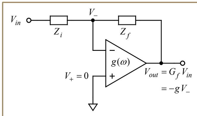
Figure 2-11: The generic inverting amplifier configuration. The op-amp has finite open-loop gain  $g(\omega)$ .  $G(\omega)$  is defined to be the gain of the circuit using an ideal op-amp;  $G_f(\omega)$  is the actual closed-loop gain.
