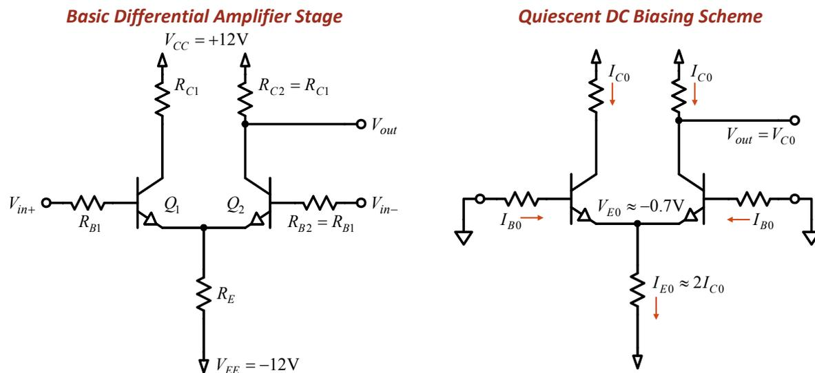
Figure 6-14: A basic *NPN* transistor differential amplifier stage, suitable for use in a simple operational amplifier design. Component and terminal identifications are shown on the left, quiescent bias currents and voltages on the right (for 0V DC inputs).
