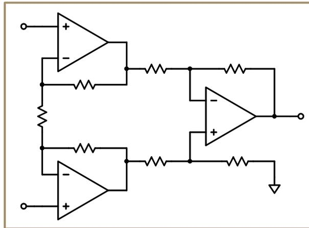
**Figure 1-32: The Instrumentation Amplifier.** This enhancement of the basic differential amplifier has a very high input impedance for both the + and - inputs, has a differential gain which can be changed by varying the value of one resistor, and has very high *common mode rejection*. It is so useful, especially for scientific applications, that many versions are available in the form of single integrated circuit devices.
