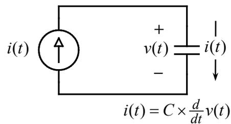
Figure 2-2 (right): A simple circuit illustrating the differential voltage-current relation for a capacitor with value  $C$ . Note the use of a *current source* to drive the capacitor in this case. Also shown are the usual conventions for the polarity of the *change in* voltage and direction of the current flow when the current  $i(t) > 0$ .
