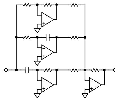
$$V_{out} = \left( k_P + k_I \int dt + k_D \frac{d}{dt} \right) V_{in}$$
