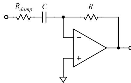
Figure 2-24: Using an input resistor to damp the differentiator.
