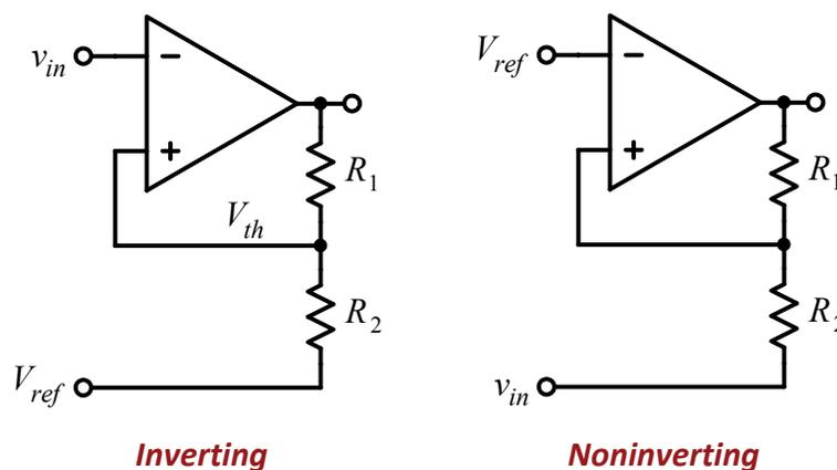
**Figure 4-4: Inverting and noninverting Schmitt triggers with a supplied reference voltage  $V_{ref}$  used to set the trigger thresholds. Note that the voltage source connected to the bottom of  $R_2$  in each circuit must have an output impedance  $\ll R_2$  or the trigger points will be affected because of the current flowing between the op-amp’s output and that source.**
