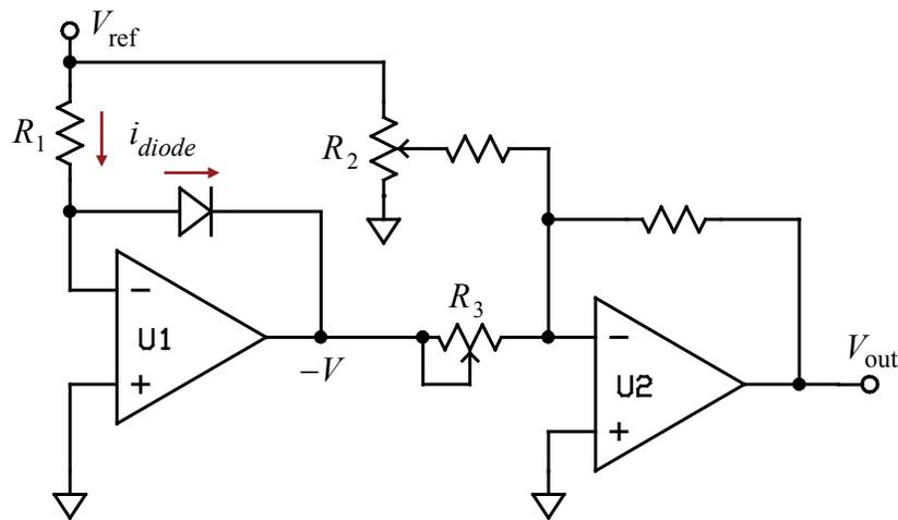
**Figure 3-8: Temperature circuit using a diode sensor. Amplifier U1 maintains a constant diode forward-bias current of  $V_{ref}/R_1$ ; the amplifier output is then  $-V$ , where  $V$  is the diode's forward-bias voltage. Amplifier U2 amplifies and offsets this voltage to provide the circuit's output ( $R_2$  trims the offset,  $R_3$  the gain).**
