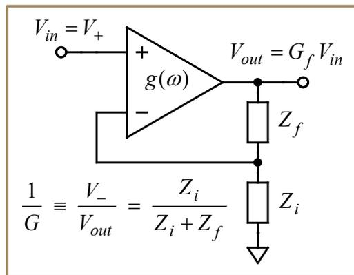
Figure 2-10: The generic noninverting amplifier configuration. The op-amp has finite *open-loop gain*  $g(\omega)$ .  $G(\omega)$  is defined to be the gain of the circuit using an ideal op-amp;  $G_f(\omega)$  is the actual *closed-loop circuit gain*.
