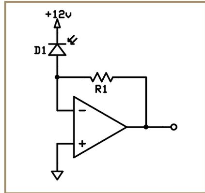
**Figure 1-30: A photodiode amplifier. The output is proportional to the light intensity; R1 sets the gain.**
