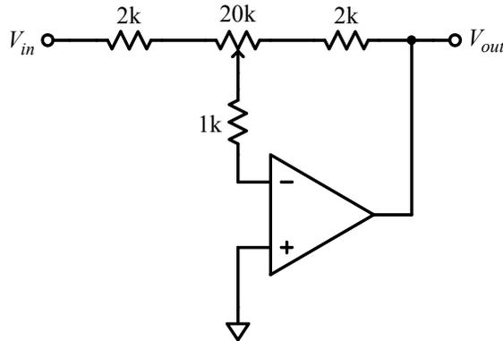
**Figure 7-2: Inverting amplifier with an adjustable gain. With the potentiometer wiper all the way to the left, the gain would be  $-22k/2k = -11$ ; wiper all the way to the right would result in a gain of  $-2k/22k = -1/11$ . This circuit will form the basis of a tone control; adding capacitors in strategic spots could make the gain adjustment only affect a subset of frequencies in the input signal.**
