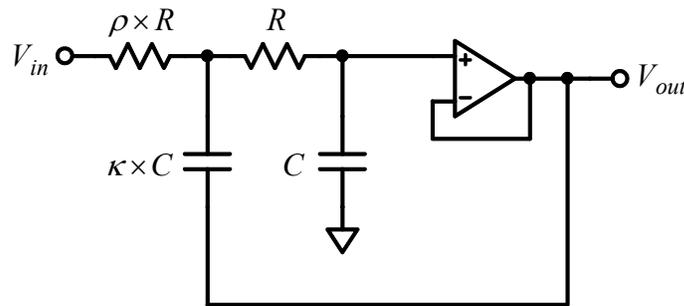
**Figure 5-19: Sallen-Key low-pass filter.** By using a voltage follower for the VCVS amplifier, the pass-band gain of the filter is unity; the ratios  $\rho$  of the resistors and  $\kappa$  of the two capacitors are chosen to select the filter's  $Q$  and resonant frequency  $\omega_0$ .
