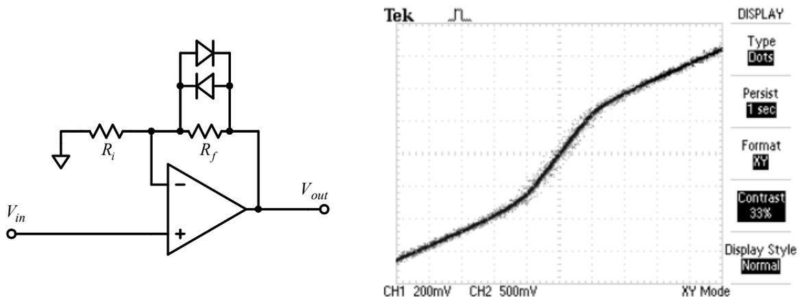
**Figure 5-20: A simple nonlinear amplifier. For large signal inputs the amplifier's *dynamic gain* drops to approximately 1, as explained in the text and as illustrated by the  $V_{out}$  v.  $V_{in}$  data shown in the right-hand image ( $R_i = 1k$ ,  $R_f = 2.2k$  for the data shown).**
