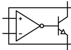
**Figure 6-10: The LM311 Comparator IC (introduced in 1969) incorporates a transistor switch with an op-amp comparator. As can be seen in the simplified functional schematic, both the output transistor's collector and emitter are accessible for incorporation into a circuit design; the output transistor is turned on (transistor collector shorted to its emitter) whenever the *-Input* voltage exceeds the *+Input* voltage.**
