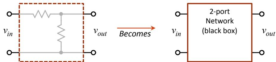
Figure 1-11: The voltage divider is a form of *two-port network*. It has a pair of input terminals, the *input port*, and two output terminals: the *output port*. In this example, the network’s transfer function (or gain function) is the ratio  $v_{out}/v_{in}$ , as already mentioned in Figure 1-7, page 1-9.
