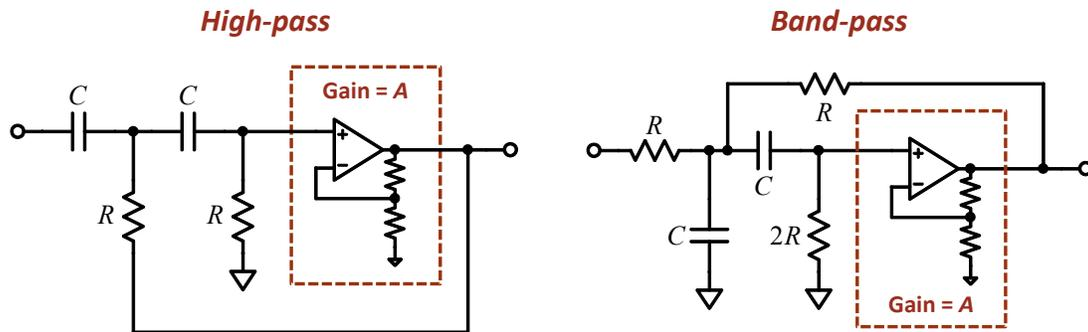
Figure 5-14: Other *VCVS* second-order filters. As with the low-pass filter, the filters'  $\omega_0 = 1/RC$ , and  $Q = 1/(3-A)$ . The in-band gain of the high-pass filter is  $A$ ; the band-pass filter's gain at  $\omega_0 = QA$ . Note that one resistor in the band-pass version of the filter has value  $2R$ .
