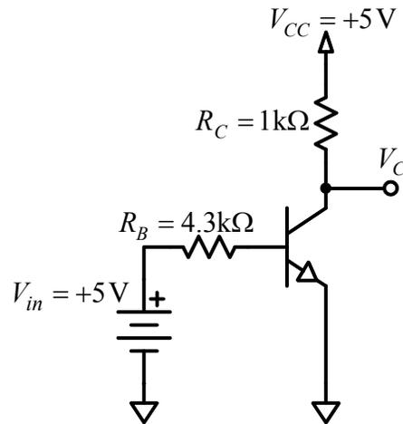
Figure 6-4: An NPN switch circuit.
