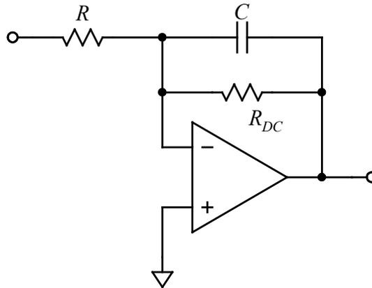
Figure 2-15: Integrator circuit. With an ideal op-amp and ignoring the action of resistor  $R_{DC}$ , then  $G(\omega) = -1/(j\omega RC)$ . In the time domain,  $v_{in}(t) = -RC (d/dt) v_{out}(t)$ , so  $v_{out}$  is proportional to the time integral of  $v_{in}$ . As explained in the text, the resistor  $R_{DC}$  limits the amplifier gain at DC so real op-amp imperfections won't cause the output to saturate.
