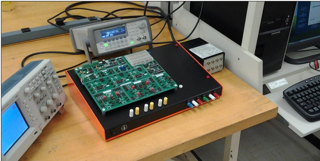
**Figure 1-25: A typical lab station setup, with analog electronics trainer and breadboard, oscilloscope, signal generator, and computer with data acquisition and control software.**
