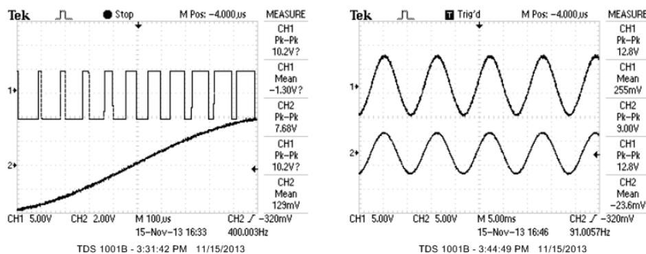
**Figure 7-5: Pulse-width modulation.** Left: the input signal level (CH2, lower trace) controls the *duty cycle* of a high-frequency, square-wave *carrier* output signal (CH1, upper trace); the *frequency* of the carrier is not affected by the input signal. Right: the *demodulated* carrier signal (CH1, upper trace) *recovers* (reproduces) the original input signal (CH2, lower trace).
