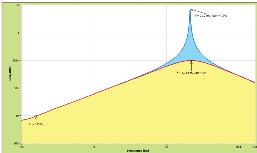
Figure 2-19: Comparison of the measured frequency responses of undamped and damped differentiator circuits ( $RC = 1\text{ms}$ ,  $C/C_{damp} = 100$ ). Data were taken using the *Frequency Response* data acquisition program. Adding the damping capacitor reduced the resonant  $Q$  from 55 to 0.75.
