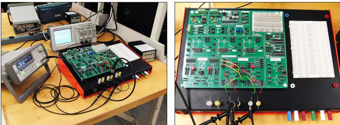
Figure 1-26: The proper way to build circuits using the breadboard's preinstalled component area.
