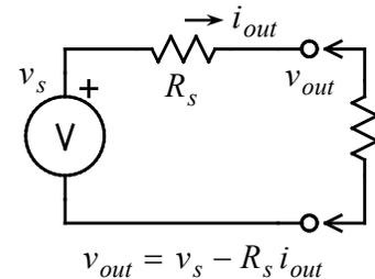
We define the output resistance of an output port in terms of the drop in the output voltage with increasing output current:
