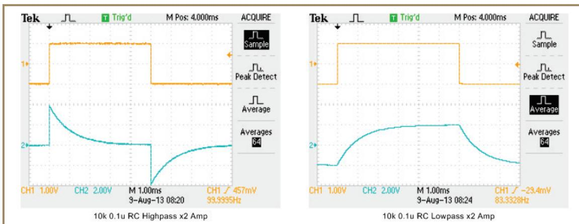
**Figure 2-9: Oscilloscope recordings of the transient responses of single-pole high-pass (left) and low-pass (right) filters to a square wave input. The  $RC$  filters' outputs were isolated and amplified by a noninverting op-amp amplifier with gain = 2. The  $RC$  time constant for both filters was 1ms.**
