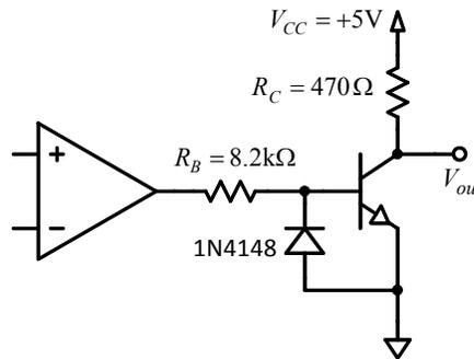
Figure 6-9: A transistor switch added to a TL082 op-amp comparator output may be used to translate the op-amp's saturated output levels of  $\pm 11\text{V}$  to the  $0\text{V}$ - $5\text{V}$  levels used by many logic circuits.
