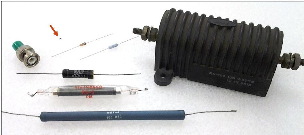
Figure 1-5: A variety of resistors, from the tiny (.08 inch × .05 inch) surface-mount component barely visible near the upper left corner of the photo (see arrow) to the beefy, 100 Watt power resistor to the upper right. The long resistor in front is designed to be used with very high voltages.
