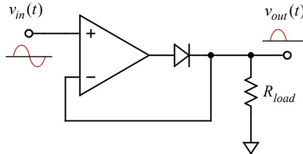
**Figure 3-4: Simple, precision half-wave rectifier. Placing the diode inside the feedback loop ensures that the op-amp output will compensate for the diode's forward voltage drop. When  $v_{in} < 0$ , the diode turns off as the op-amp output goes negative;  $R_{load}$  then ensures that  $v_{out} = 0$  in this case.**
