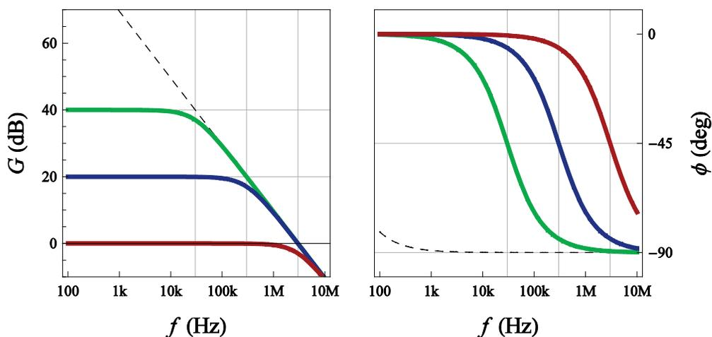
Figure 2-13: Bode plots of noninverting amplifiers with closed-loop gains of 100 (Green), 10 (Blue), and 1 (Red). The  $-3\text{dB}$  corner frequencies are at  $f_{BW}/G_{DC}$ . Also shown (dashed) are the TL082 op-amp open-loop gain and phase using the simplified model given by (2.18).
