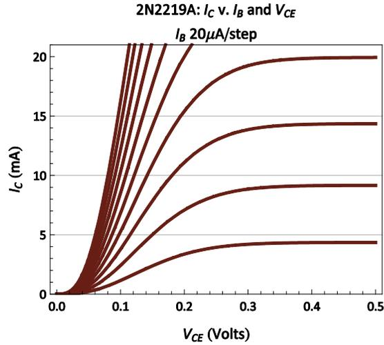
Figure 6-5: Saturation region of the transistor characteristic curves. The left-most curve corresponds to  $I_B = 0.2$  mA; note that even this relatively small base current will drive the collector-emitter voltage drop down to only about 0.1V even for collector currents as high as 20mA.
