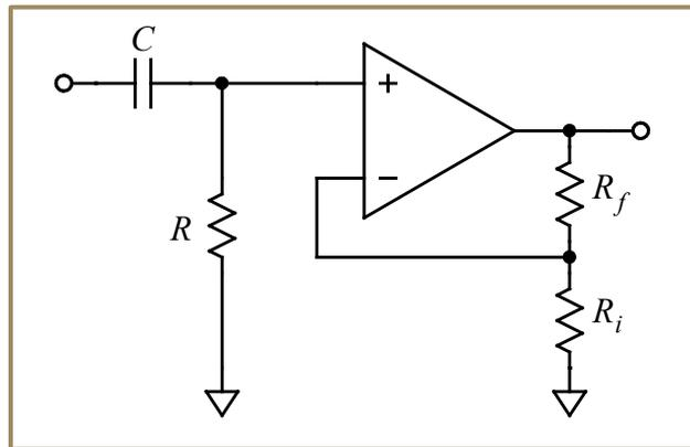
**Figure 2-8: Using AC coupling to prevent unwanted amplification of the DC component of the input. The low-frequency cutoff of the amplifier is determined by the filter's RC corner frequency,  $f_0 = 1/(2\pi RC)$ . The gain within the passband is determined by the amplifier's feedback resistors:  $G = 1+(R_f/R_i)$ . The input impedance of the amplifier (in the passband) is  $R$ .**
