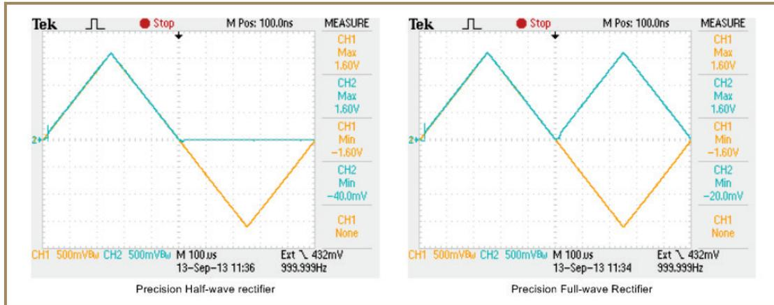
**Figure 3-6: Precision rectifier outputs. Left: half-wave rectifier circuit of Figure 3-4. Right: full-wave rectifier of Figure 3-5. Input signal waveform and display scales are the same as in Figure 3-3 on page 3-4; note that the precision rectifier circuits eliminate the 0.6V forward voltage drop of the silicon diode used in the circuits. The small “glitches” in the output waveforms as the input goes through 0 are effects of the TL082 op-amp’s finite slew rate.**
