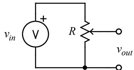
Figure 1-9 (right): A potentiometer with total resistance  $R$  used as a variable voltage divider. As the wiper position is adjusted from bottom to top,  $v_{out}$  varies from 0 to  $v_{in}$ .
