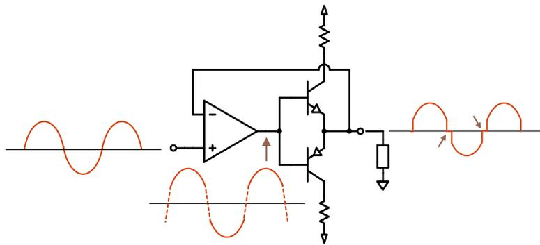
Figure 6-17: Generation of *crossover distortion* in the simple, *Class B* power-booster’s output caused by the transistors’ 0.7V base-emitter turn-on voltage coupled with the op-amp’s finite slew rate.
