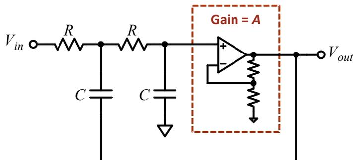
Figure 5-13: A simple version of the *VCVS* second-order, active low-pass filter, in which both the resistors and the capacitors of the two cascaded *RC* filters are chosen to be equal. The non-inverting op-amp amplifier stage has gain  $A$  (if a simple voltage follower is used, so  $A = 1$ , then the circuit is called a *Sallen-Key* filter). The circuit's resonant frequency is  $\omega_0 = 1/RC$ , and its  $Q = 1/(3-A)$ . The circuit's in-band gain is  $A$ .
