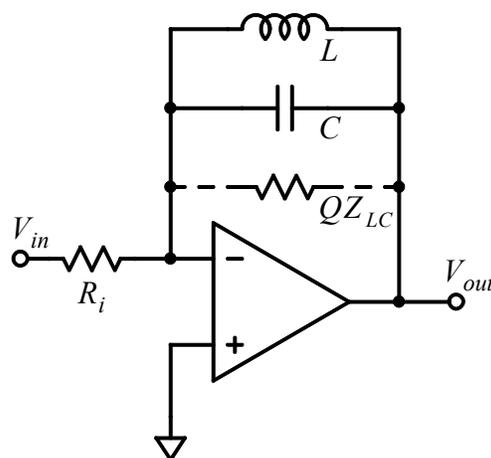
**Figure 5-1:** An inverting amplifier with a parallel  $LC$  combination forming the feedback impedance. In addition the circuit will include an equivalent parallel resistance along with the  $L$  and  $C$ . Its equivalent value  $QZ_{LC}$  is addressed in the text.
