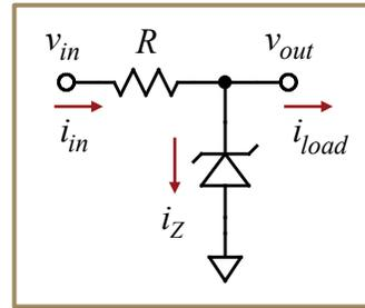
**Figure 3-18: Zener diode voltage regulator circuit. The input voltage  $v_{in}$  must be greater than the Zener diode's reverse breakdown voltage,  $V_R$ . This large voltage causes the diode to suffer reverse breakdown, with the difference  $v_{in} - V_R$  imposed across resistor  $R$ , establishing the input current  $i_{in}$ . This current is divided between that required by the load,  $i_{load}$ , and the reverse current through the diode,  $i_Z$ .**
