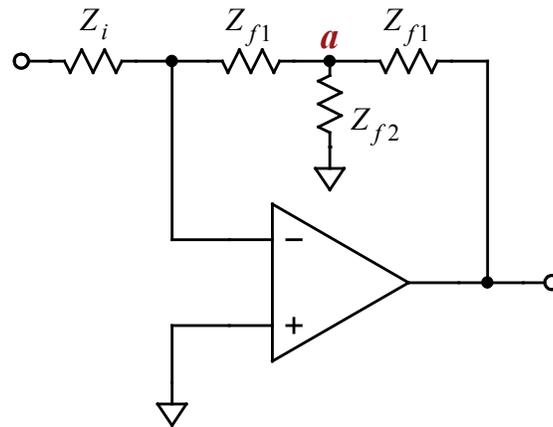
**Figure 2-26:** A high gain inverting stage which doesn't require a small value for the input impedance,  $Z_i$ . The current through  $Z_i$  also flows through the left-hand  $Z_{f1}$ , so the voltage at node **a** is  $-(Z_{f1}/Z_i)V_{in}$ . But the voltage at this node must be a weighted sum of the voltages at other ends of the impedances joined to it, two of which are 0, so also solving for  $V_a$  in terms of  $V_{out}$  gives the gain equation 2.24.
