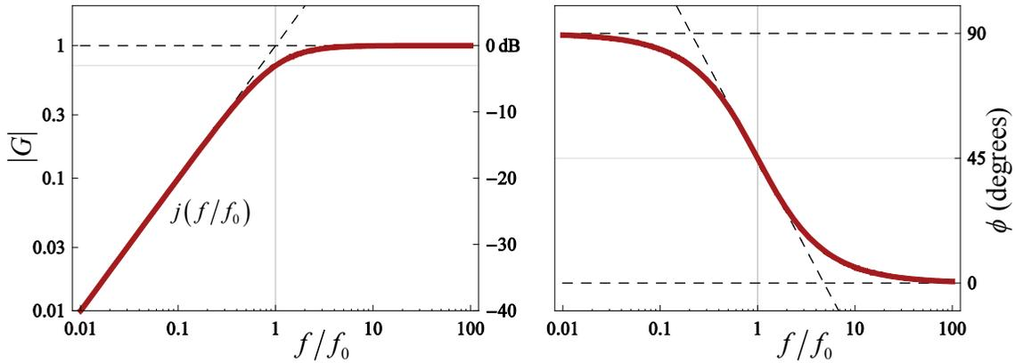
Figure 2-7: Bode plot of the RC high-pass filter response from equation 2.12. The asymptotes of the response are shown as dashed lines. Frequency is relative to the RC corner frequency,  $f_0 = 1/(2\pi RC)$ , as in Figure 2-5. Gain is also shown in decibels (dB):  $G(\text{dB}) = 20 \log_{10}(G)$ . This response is typical of that of a *single pole filter*.
