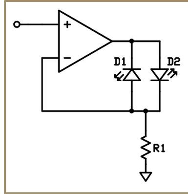
Figure 1-31: A LED driver using a transconductance amplifier. LED  $D1$  is illuminated for  $V_{in} < 0$ ,  $D2$  whenever  $V_{in} > 0$ . Resistor  $R1$  sets the conversion from input voltage to LED intensity.
