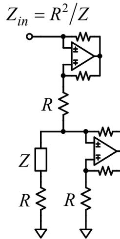
A more sophisticated application of combined positive and negative feedback to implement a gyrator circuit is shown in Figure 5-7. This circuit is quite different from the negative impedance circuit, and it is quite stable, though we won't consider its stability in detail here.
