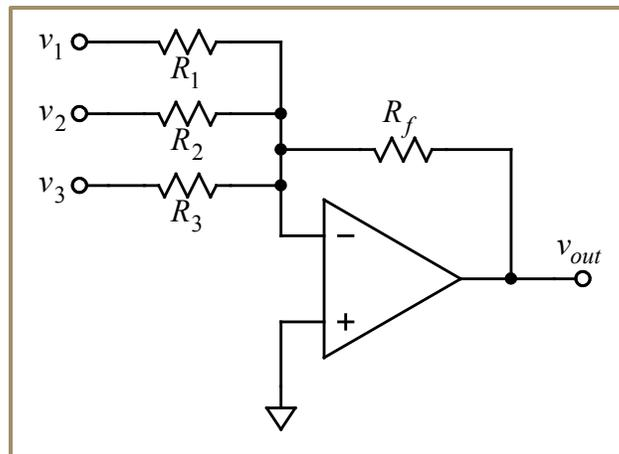
**Figure 1-21: The inverting, Summing Amplifier.** The node joining the resistors to the *-Input* is a *virtual ground*, so each input will be amplified independently of the others. The result is a weighted sum of the several inputs (inverted, of course) given in equation 1.9.
