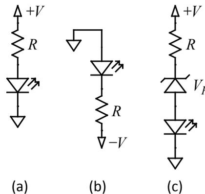
**Figure 3-19: LED pilot light circuits. (a) positive supply voltage; (b) negative supply voltage; (c) positive voltage, but with a minimum voltage threshold for LED illumination using a Zener diode. See the text for details.**
