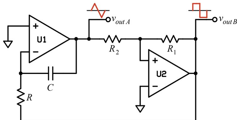
Figure 4-6: Integrator coupled to a Schmitt trigger to form a primitive *function generator*, outputting triangle and square waveforms. Since the integrator is inverting, its output must go to a noninverting Schmitt trigger, so that reaching a trigger point reverses the capacitor's charging current. This means that we must have  $R_1 > R_2$ , or the circuit won't work.
