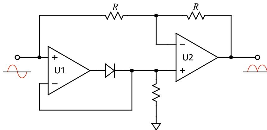
**Figure 3-5: Precision full-wave rectifier. The output of a half-wave rectifier is combined with the original input signal by the amplifier U2. Its output is the absolute value of the input. The two resistors  $R$  should be well-matched in value (1% or better).**
