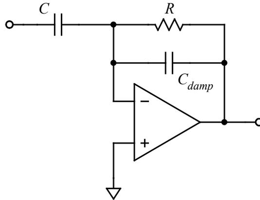
Figure 2-17: Differentiator circuit. With an ideal op-amp and ignoring the action of capacitor  $C_{damp}$ , then  $G(\omega) = -j\omega RC$ . In the time domain,  $v_{out}(t) = -RC (d/dt) v_{in}(t)$ . As explained in the text, the capacitor  $C_{damp}$  dampens response overshoot and “ringing” following a step input caused by a real op-amp’s limited frequency response.
