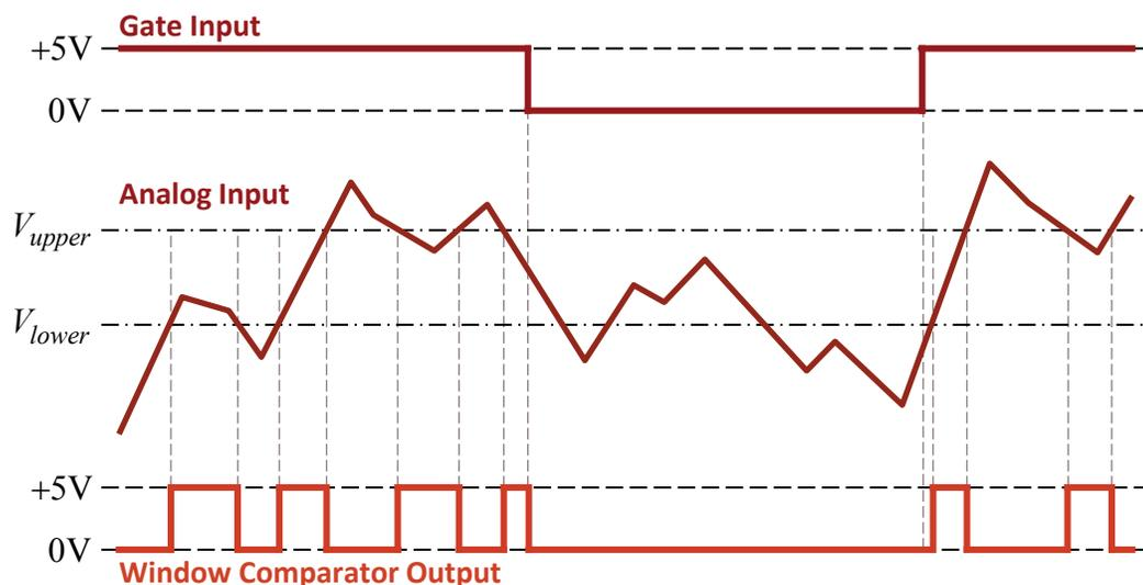
Figure 7-4: Sample *window comparator* behavior. The comparator's output is active only while its *Gate* input is high (or disconnected). When active, the comparator's output is high whenever its analog input signal voltage falls within the window defined by two adjustable thresholds,  $V_{lower}$  and  $V_{upper}$ .
