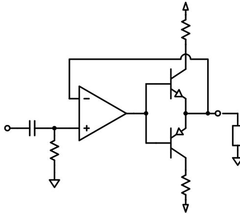
**Figure 6-16:** A simple *push-pull* emitter follower circuit uses a *complementary pair* (*NPN* and *PNP*) of transistors to boost the output current of an op-amp. Note that the negative feedback is from the transistors' output (the little hump in the feedback wire as it crosses below the resistor means that there is no connection between the crossing wires). The collector resistors reduce the transistors' power dissipation when driving a low-resistance load.
