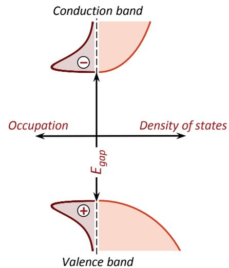
**Figure 3-20: Densities of states and occupations by electrons (conduction band) and holes (valence band) for a pure semiconductor (only intrinsic charge carriers); energy increases in the vertical direction. The kinetic energy distribution of the charge carriers in each band is classical.**
