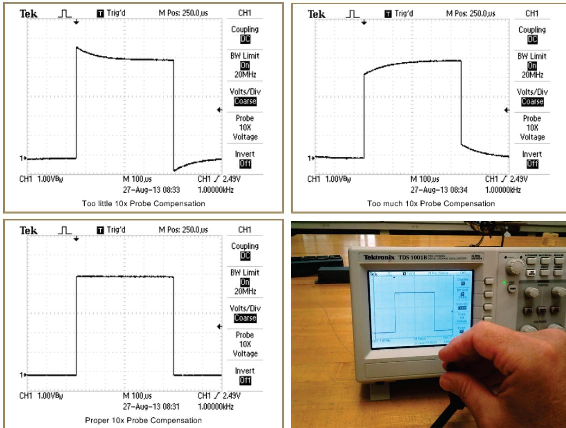
Figure 2-27: Properly adjusting the 10x probe compensation. The probe and its ground are clipped to the 1kHz signal output provided on the oscilloscope front panel. Using the special tool provided specifically for this purpose, the user carefully adjusts the probe's internal capacitor until the displayed waveform is as flat as possible, as shown in the lower left image. The upper images show outputs when the probe is not properly compensated.
