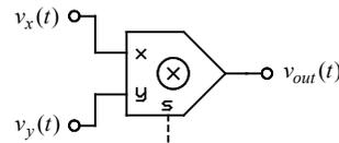
The analog multiplier usually has a precision, built-in scale factor which is often  $s = 10.0V$ , but it may include an external terminal so that you can adjust the value of  $s$  (as shown in the schematic above). However the scale factor may be set, it is usually limited to positive values ( $s > 0$ ). Modern analog multipliers don't limit the signs of  $v_x$  and  $v_y$  (they support "four-quadrant multiplication"), but they may limit their magnitudes to  $\leq s$ .
