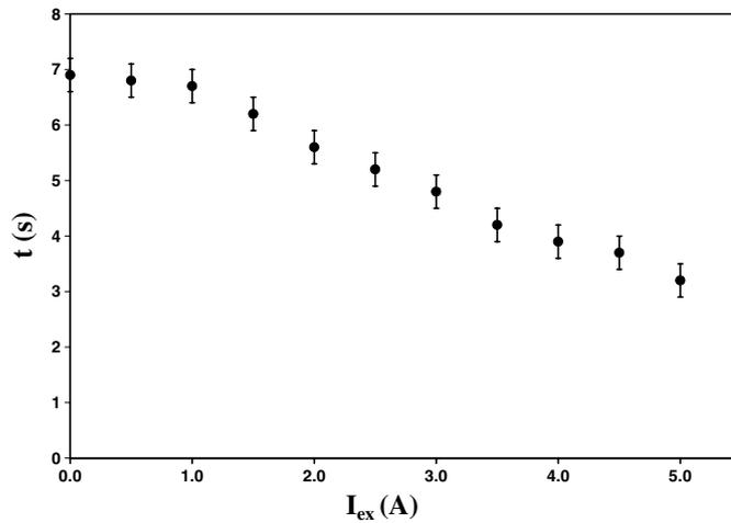
**Figure 3.** Braking time for the copper disc versus excitation intensity. The initial speed of the disc was set to 200 rpm.
