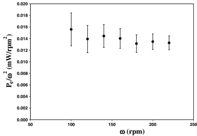
**Figure 4.** An example to test the proportionality between  $P_e$  in the copper disc and  $\omega^2$ . The excitation intensity was fixed to 3.0 A.
