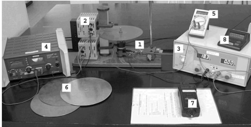
**Figure 2.** The whole experimental setup. 1: dc motor with one of the discs attached to it. 2: Electromagnet. 3: dc power source for the motor with built-in voltmeter. 4: dc power source for the coil with built-in ammeter. 5: Ammeter for the motor. 6: Discs of other materials. 7: Optical tachometer. 8: Stopwatch (photograph courtesy F Herrera).
