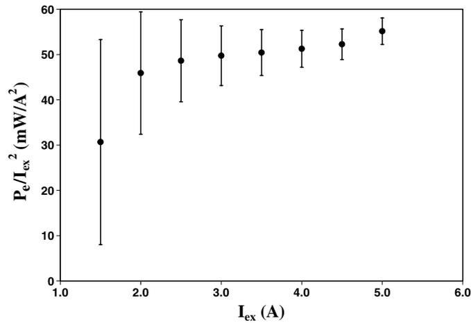
**Figure 5.** An example to test the proportionality between  $P_e$  in the copper disc and  $I_{ex}^2$ . The angular speed was fixed to 200 rpm.
