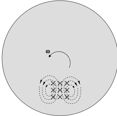
**Figure 1.** A sketch of the eddy currents in a rotating disc. The crosses represent a steady magnetic field perpendicular to the plane of the disc. According to Faraday's law, eddy currents appear in those points of the disc where the magnetic field increases or decreases.
