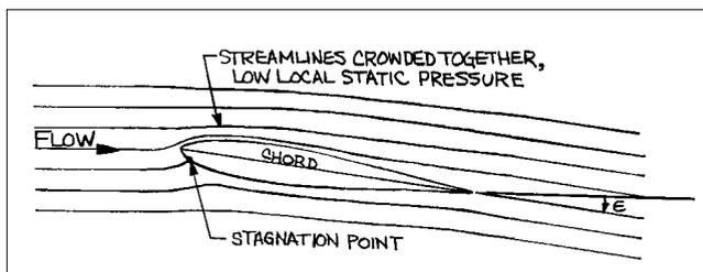
Fig. 4. Symmetric airfoil at positive angle of attack.
