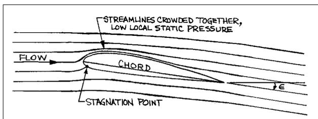
**Fig. 2. Streamlines around the NACA 2412 airfoil.**
