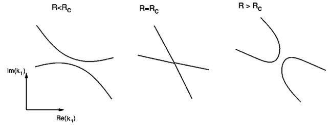
FIG. 1. Bifurcation of the solutions of the boundary equations at  $(k_1^c, k_0^c, R^c)$ . The curves represent the trace of  $k_1$  as a function of  $\omega$  for three different values of the reflectivity  $R$ .
