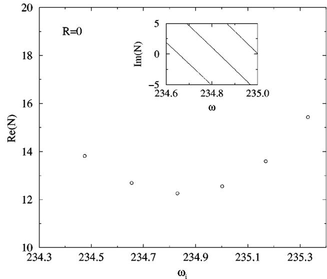
FIG. 3. Carrier density vs frequency for the laser without external mirror. Inset: the frequencies of the monochromatic modes correspond to the intersection of the lines  $\text{Im}[N(\omega)]$  with the  $\omega$  axis. The frequencies are measured in units of  $1/T$ .
