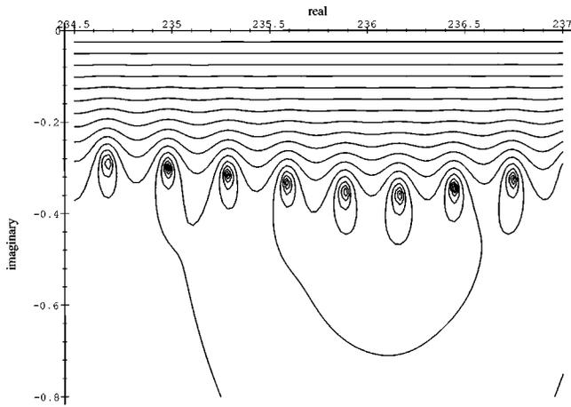
FIG. 2. Complex wave vector  $k_1$  allowed for different values of  $R$ . Contour lines are labeled by  $R$  and increase from  $R=0$  (points) to  $R=1$  (real axis).
