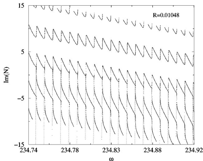
FIG. 6. Function  $\text{Im}[N(\omega)]$  for  $R=0.01048$ . Different lines correspond to different determinations of  $k_1(\omega)$ . The points with  $\text{Im}[N(\omega)]=0$  correspond to solutions of the problem.
